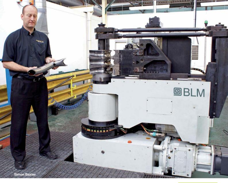
end of the tube prior to bending. End forming tools for other diameters and forms of breather pipe can be premounted if required, thereby eliminating non-productive changeover time, while the mounting of different diameter tooling on the Dynamo tube bender also eliminates downtime when changing from one size of tube to another. With a cycle time typically of 1.5 seconds per bend, CTC is confident that it has now achieved the highest possible output while maintaining optimum repeatability.
